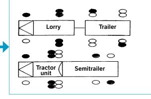
Note: Chains have to be re-tensioned after driving about 100–200 metres.
