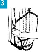
First, hook up the side chains on the inner side of the wheel.
