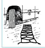
Positioning may vary in vehicles with ABS and EBS. Chains must be fitted on wheels with ABS sensors. (See the instruction manual.)
